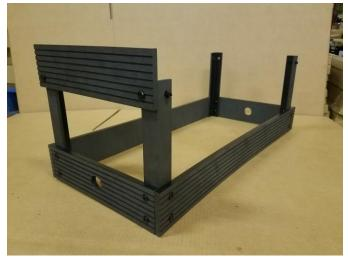
Next attach the remaining panels in a clockwise manner. The panels will attach above the corner brace edges, not flush.
