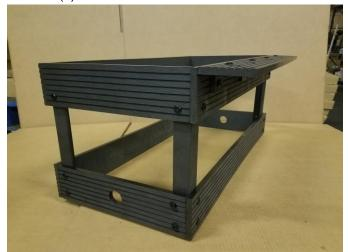
Align and square each corner of the frame and then fully tighten the screws.
