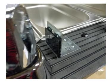
Remove the film from the Velcro backing, and attach to the provided splash guard (also with the film peeled back).
