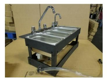
Remove the pans, and lay a thin bead of Silicone around the entire top edge of the sink pan frame. Reinsert the pans and align as desired, then place 20-30lbs of pressure across the top and allow the Silicone to fully cure.
